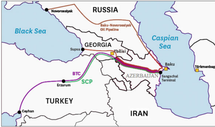
Fig. 3.19 The South Caucasus pipeline. Source http://www.socar-germany.de/eng/socar/scp.html
