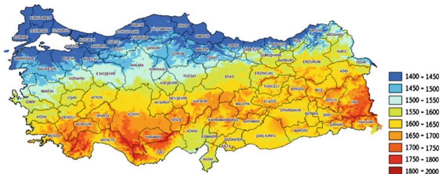
Fig. 4.4 Solar radiation map of Turkey (annual kWh/m 2 ). Source EIE http://www.eie.gov.tr/MyCalculator/Default.aspx (Accessed on December 19, 2011)
