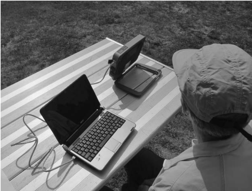
Figure 7.1 Battery operated Inmarsat satellite data terminal.
