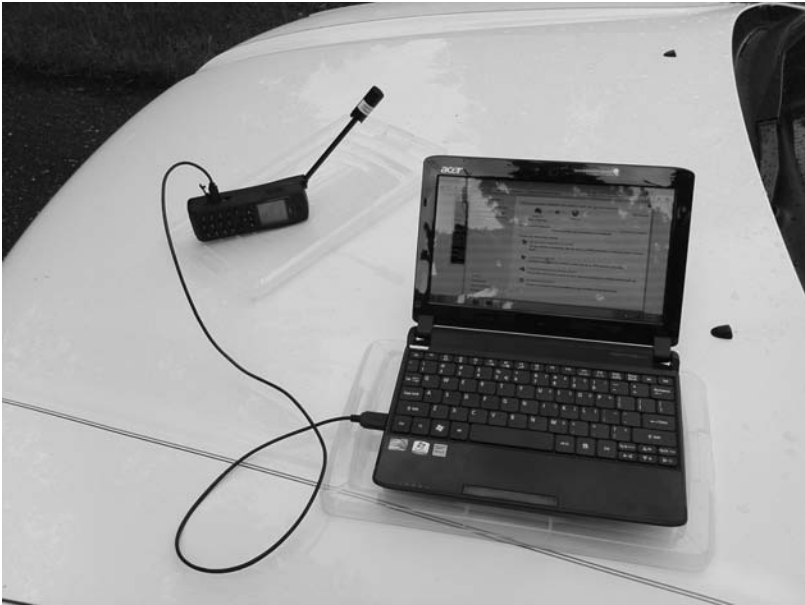
Figure 7.2 Internet connection for (slow) data through iridium satellite phone.
