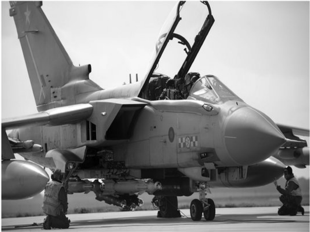
A RAF Tornado GR4 on the ground showing the mix of Paveway and Brimstone missiles. (Crown Copyright)
